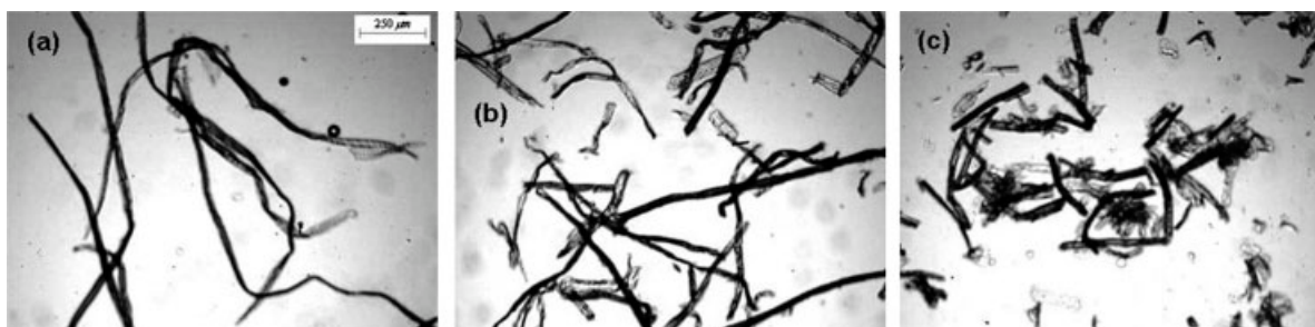
Figure 3 Microscopic images for (a) no treatment, (b) 60 min, and (c) 240-min high-dosage cellulase treatments. Scale bar shows 250 \mu\text{m} in (a).
